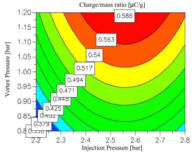
Fig. 6. Contour plot of the response predicted by the quadratic model: variation of the charge/mass ratio when the injection and vortex pressures vary over the range defined by the experimental design, at  $p_{dil} = 1.7$  bar.
