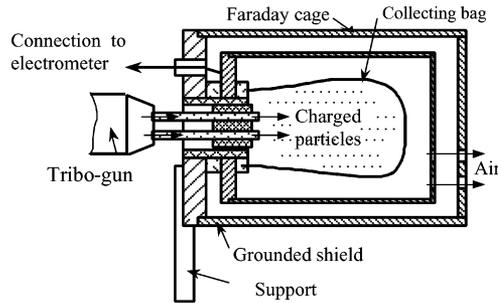
Fig. 3. Custom-designed Faraday pail for powder charge measurements.
