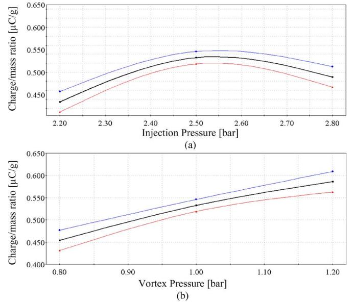
Fig. 5. Plot of predicted response and the 95% confidence interval, as function of the injection pressure, for (a)  $p_{dil} = 1.7$  bar and  $p_{vor} = 1$  bar, and as a function of the vortex pressure, for (b)  $p_{inj} = 2.5$  bar and  $p_{dil} = 1.7$  bar.
