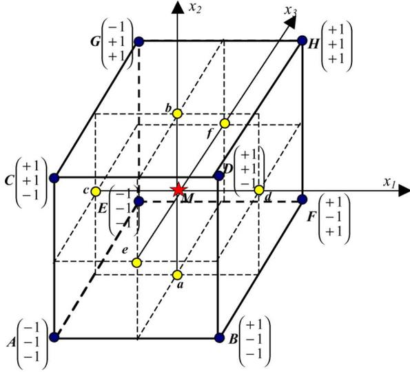
Fig. 1. Representation of the 17 experimental points of the composite design.
