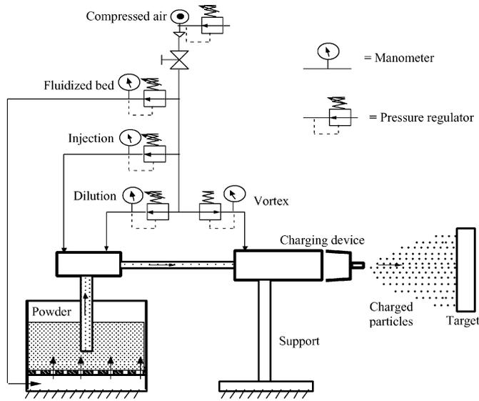
Fig. 2. Schematic representation of the powder tribocharging installation.
