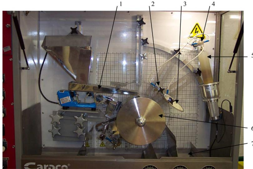
Fig. 1. Roll-type corona electrostatic laboratory separator (CARPCO Inc., Jacksonville, FL) with high-voltage probe. 1: feeder; 2: corona electrode; 3: electrostatic electrode; 4: high-voltage connector; 5: high-voltage probe; 6: grounded roll electrode (carrier); 7: collector.
