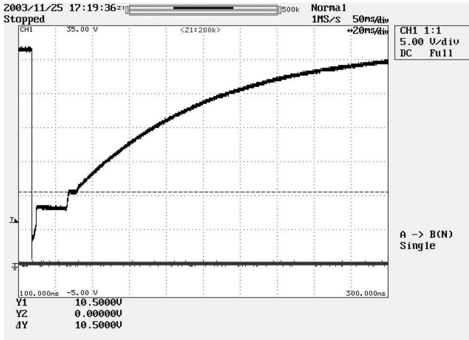
Fig. 8. Voltage restoring curve for the HV supply #1, as displayed by the oscilloscope, at 5 kV/div and 20 ns/div.
