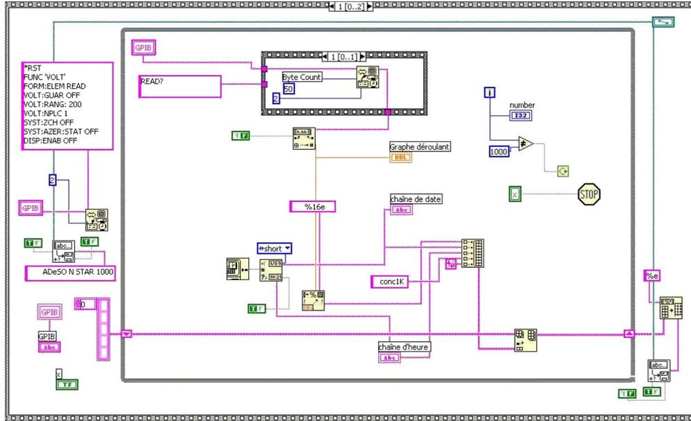
Fig. 3. Diagram of the virtual instrument employed for HV monitoring, using a HV probe and a digital electrometer.
