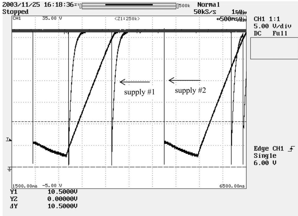
Fig. 7. Voltage restoring curves for the two HV supplies obtained with the digital oscilloscope (5 kV/div, 500 ns/div). The graph resulted from the superposition of the curves recorded for two series of spark discharges, one for each of the HV supplies.
