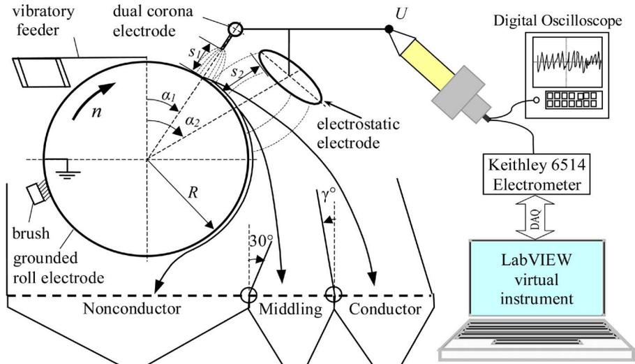
Fig. 2. Experimental setup for HV monitoring using: a high-voltage probe (model PVM-5, NorthStar Research); a digital electrometer (model 6514, Keithley) with a virtual instrument developed in a LabVIEW environment; and a digital oscilloscope (model DL1740, Yokogawa).
