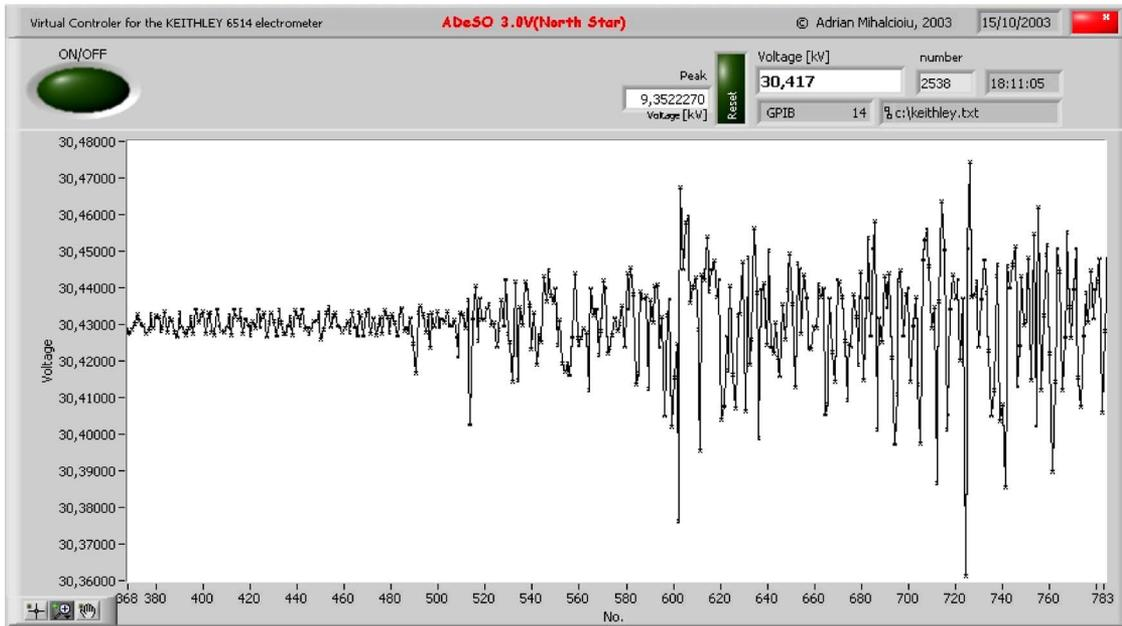
Fig. 4. HV variation before and during granular-material processing, as displayed by the virtual instrument developed in LabVIEW.
