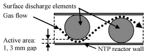
Fig. 4. Testing active area setup for surface discharge elements.
