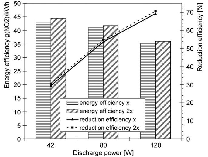
Fig. 7. Comparison of energy and reduction efficiency for a distance between surface discharge elements of  $x = 70$  mm and  $2x = 140$  mm.
