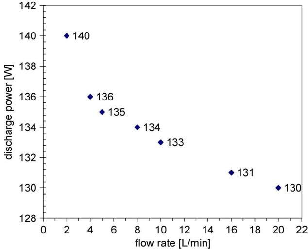
Fig. 6. Influence of gas flow rate on discharge power (each point is the average value of five measurements).
