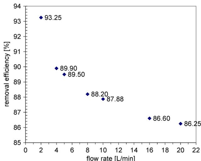
Fig. 5. Reduction efficiency of NO 0.04 [L/min] diluted in N<sub>2</sub> at various flow rates (average values of five measurements).
