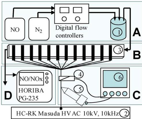
Fig. 2. Schematic representation of the experimental setup: (1) Gas mixing chamber; (2) HC-RV Masuda Research HV supply; (3) Plasma reactor; (4) Tektronix P6021 current probe; (5) IWATSU HVP60 HV probe; (6) Yokogawa DL1740 digital oscilloscope.
