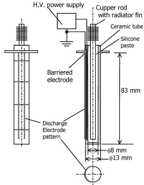
Fig. 3. Surface discharge element for NTP reactor.
