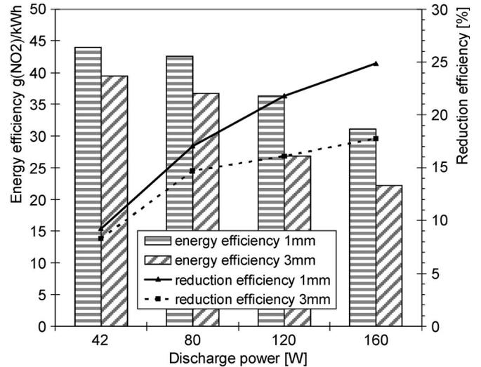
Fig. 8. Comparison of energy and reduction efficiency for 1- and 3-mm gap.
