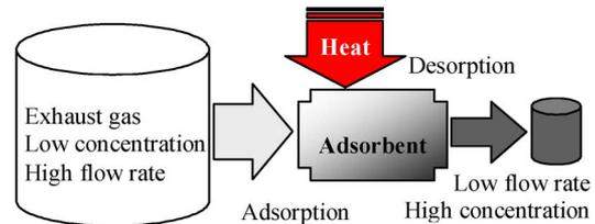
Fig. 1. Concept of concentrating exhaust gas using adsorption and thermal desorption.
