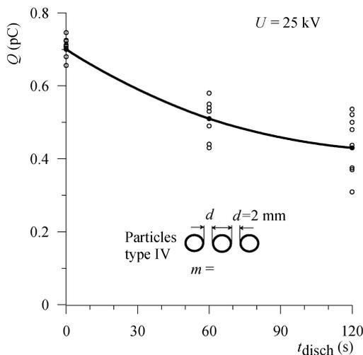
Fig. 8. Charge  $Q$  of type-IV particles as function of discharging time  $t_{\text{disch}}$  (the conditions of the experiment are similar to those in Fig. 7).
