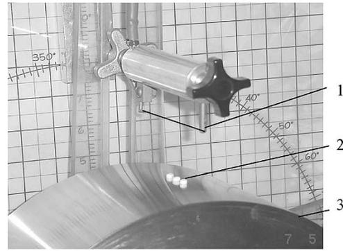
Fig. 3. (a) Schematic representation of the four types of particles employed in this experiment and (b) view of the corona charging experimental setup. 1: corona electrode; 2: charged particles; 3: grounded roll electrode.
