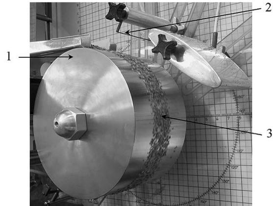
Fig. 1. Charged insulating particles “pinned” on the surface of the grounded electrode of a roll-type corona electrostatic separator. 1: grounded rotating roll electrode; 2: corona electrode; 3: charged particles.
