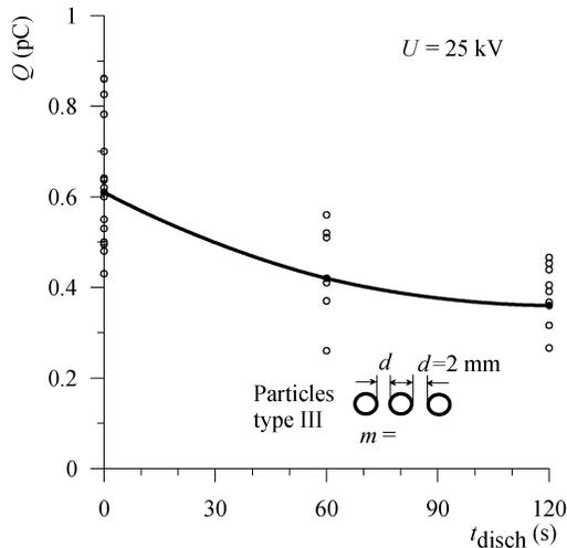
Fig. 7. Charge  $Q$  of type-III particles as function of discharging time  $t_{\text{disch}}$  (the particles were charged by groups of three, for a spacing  $d = 2$  mm, at  $V = 25$  kV, and  $s = 50$  mm; the represented points are average values computed by dividing the measured charge by the number of particles collected in the Faraday pail).
