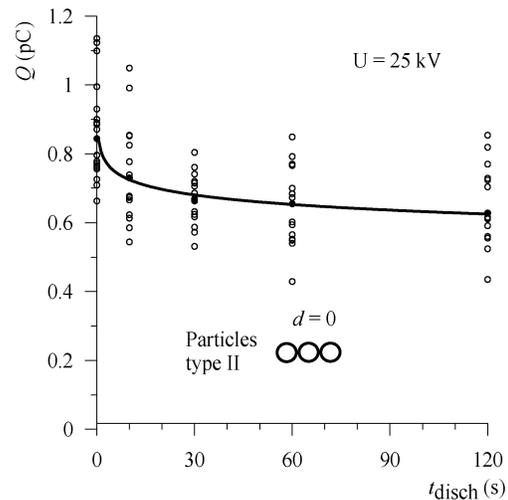
Fig. 6. Charge  $Q$  of type-II particles as function of discharging time  $t_{\text{disch}}$  (the particles were charged by groups of three, for a spacing  $d = 0$  mm, at  $V = 25$  kV, and  $s = 50$  mm).
