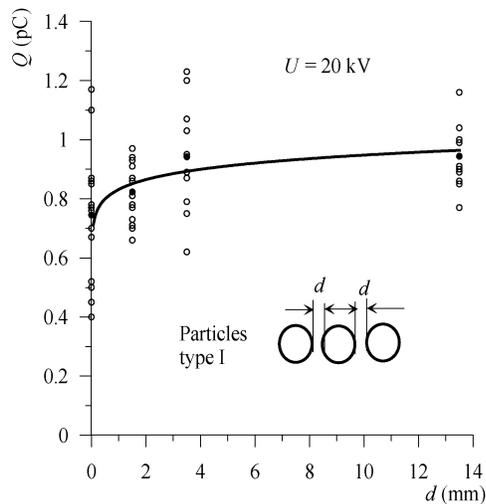
Fig. 4. Charge  $Q$  of type—I particles as function of spacing  $d$ , for an applied voltage  $V = 20$  kV, and a distance  $s = 50$  mm between the electrodes.
