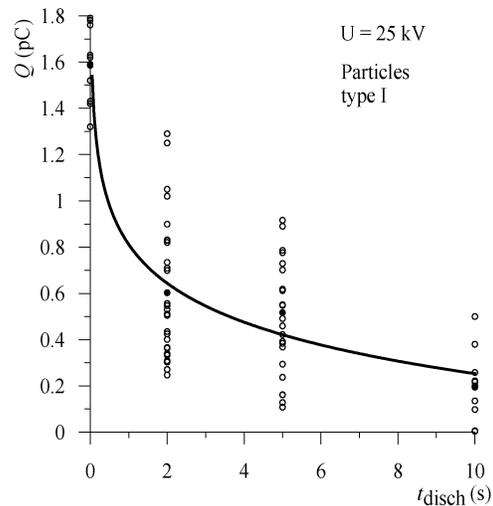
Fig. 5. Charge  $Q$  of type-I particles as function of discharging time  $t_{\text{disch}}$  (the particles were individually charged at an applied voltage  $V = 25$  kV, and a distance  $s = 50$  mm between the electrodes).
